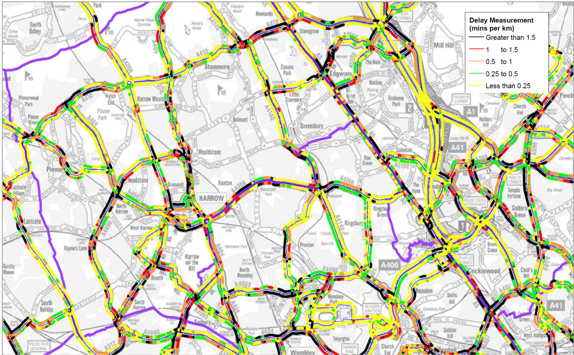
Figure A.2: May 2009 Average Delay – PM peak period 4 pm to 7 pm (working days only Mon to Fri)
