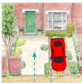
Paved tracks Loose gravel
