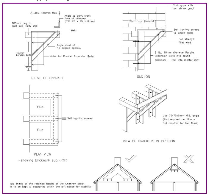
The use of Gallows Brackets is **NOT** permitted on a Party Wall if the chimney on the other side of the wall has previously been removed and is supported on Gallows Brackets. See Beam Support Detail.
